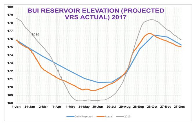
Figure 3: Bui Reservoir Trajectory (Actual)
