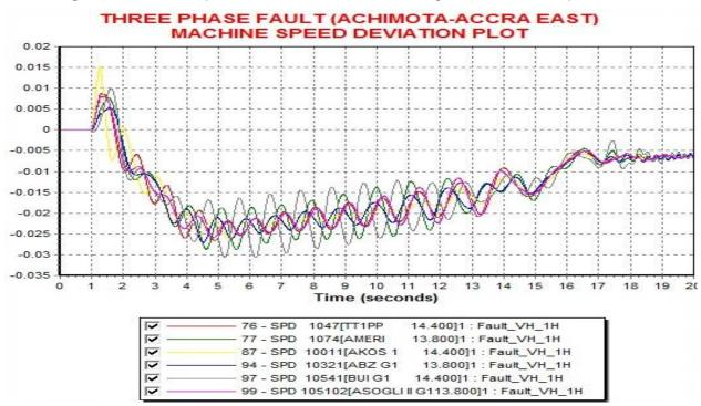
Figure 13: Case 1 - Speed deviation of machines on the grid for 161kV three phase fault
