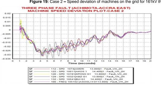
Figure 19: Case 2 - Speed deviation of machines on the grid for 161kV three phase fault
