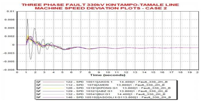
Figure 24: Case 2 - Speed deviation of machines for a 330kV three phase fault in the north
