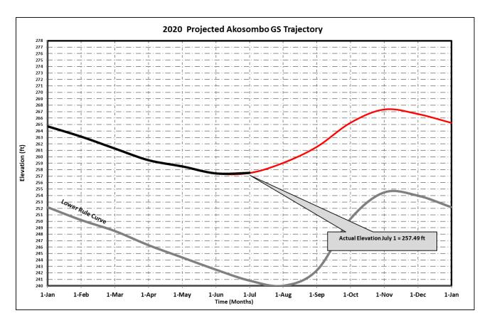
Figure 4.1: 2020 Projected Akosombo Reservoir Trajectory
