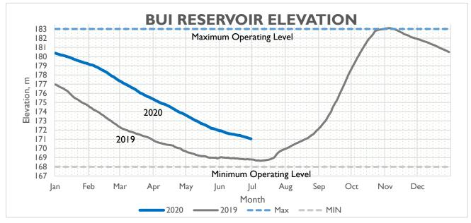
Figure 2.8: Bui Reservoir Trajectory
