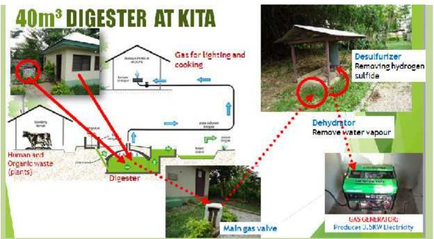
Plant layout of biogas plant at KITA
