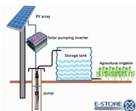
Demonstration of Solar Pumping System for crop irrigation
