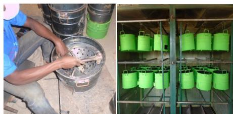
Assembling of Combustion Chamber and Body (top left) and Oven-drying of Sprayed Stove (top right); Cookmate Coal Pot (bottom)
