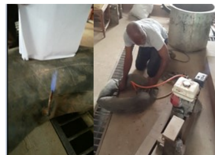
From left, Blue Gas Flame; next, Two Stroke ICE being Powered by the Gas Generated from the Pyrolysis Process (Photo credit: Fritzi Ziebel and Eugene Sefa-Appiah)
