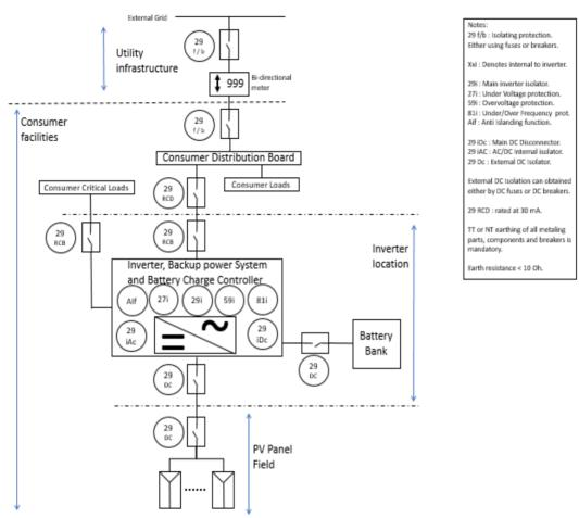
Figure 3: Renewable Energy Generating Facility connection to the Low Voltage Distribution Network.
