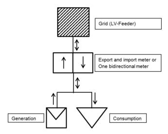
Figure 2: Metering Configuration for Bi-directional Net Metering
