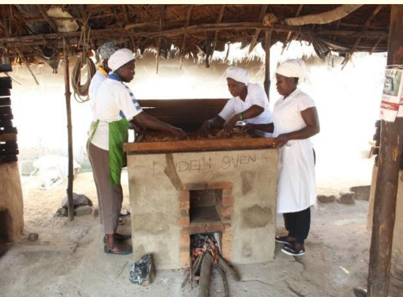
Figure 27: Ahotor oven being used to smoke shrimps at Akplorworkor
