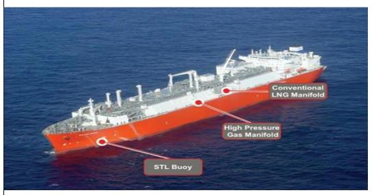
Figure A3. LNG Energy Bridge Regasification Vessel
