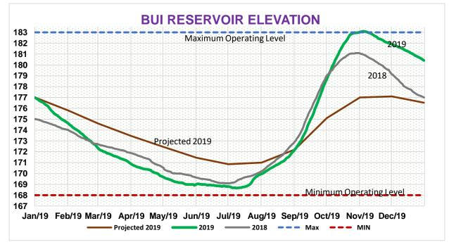
Figure 2: Bui Dam reservoir trajectory in 2019
