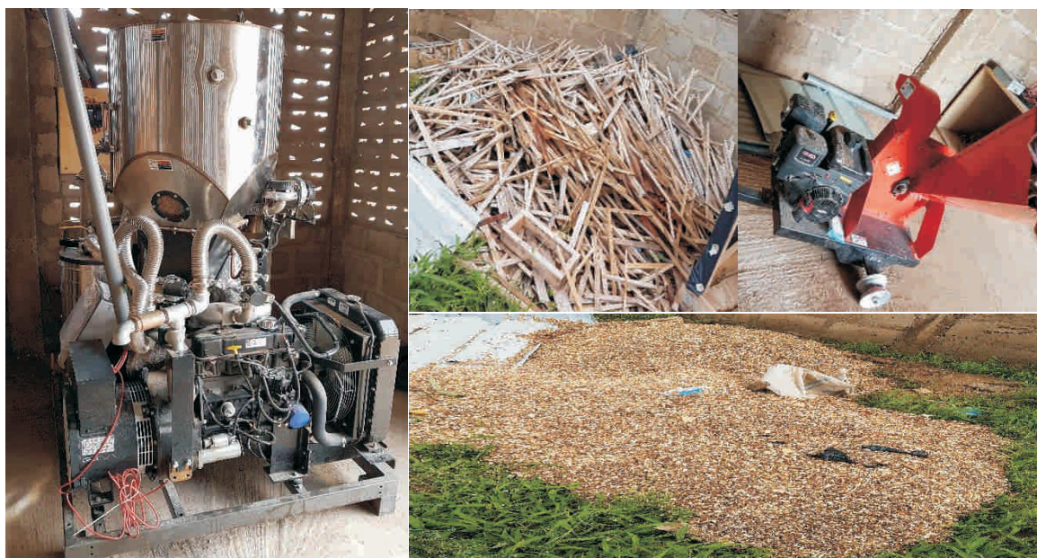
Left: 20 kW gasifier. Right: Wood off-cuts from the timber market cut into chips with a chipping machine
