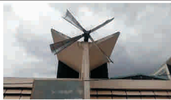
Figure 39: 100kW wind turbine Prototype
