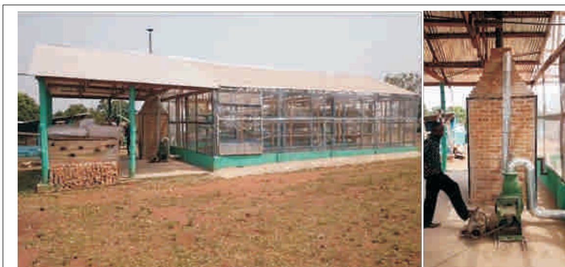
Figure 19: Solar-biomass hybrid dryer at the Ejura market
