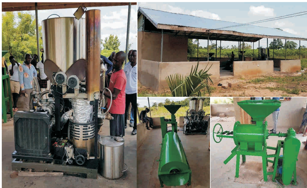
Left: 20 kW gasifier. Right: Palm oil processing centre with nut cracker and palm oil expeller
