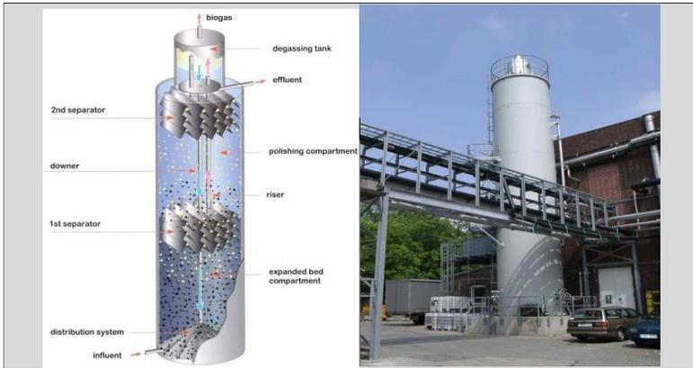
Internal Circulation Anaerobic Reactor
