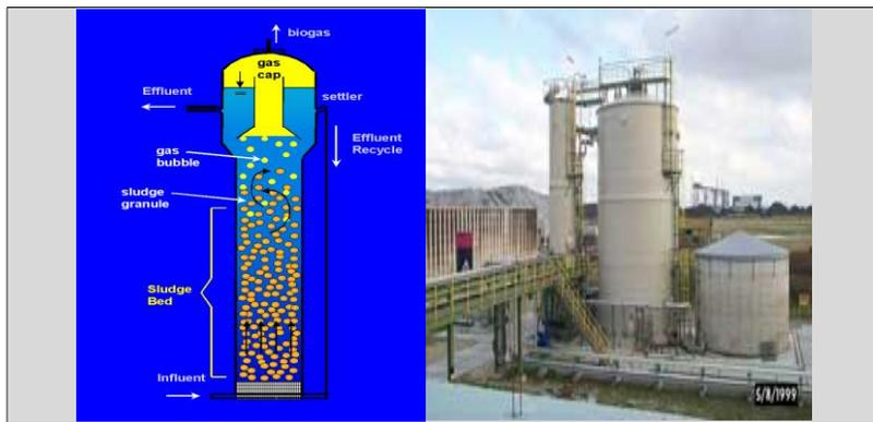
Expansion Granular Sludge Bed Reactor
