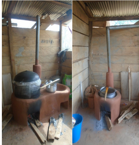
A double and single chamber improved mud stove with chimney constructed by Trees for the Future
