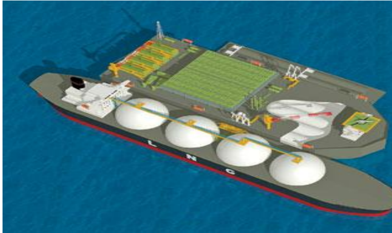
Figure A4. LNG Floating, Storage And Re-Gasification Plant
