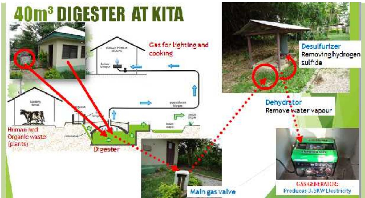
Plant layout of biogas plant at KITA
